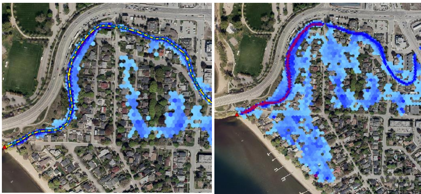
Figure 6-5: 5-year Lake Level (left) with 200-year Mill Creek Flows and 2017 Lake Level (right) with 200-year Flows
