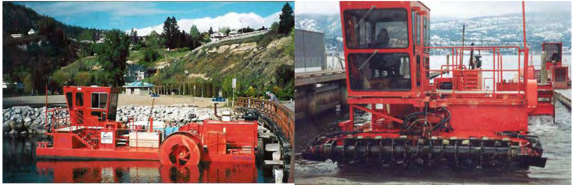
Figure 4: Rototiller from side, showing paddlewheels toward bow and enclosed cab at stern and rototiller from rear showing rototiller blades at stern of machine
