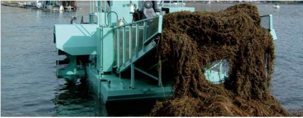
The machine used for harvesting Eurasian watermilfoil from Okanagan lakes.
