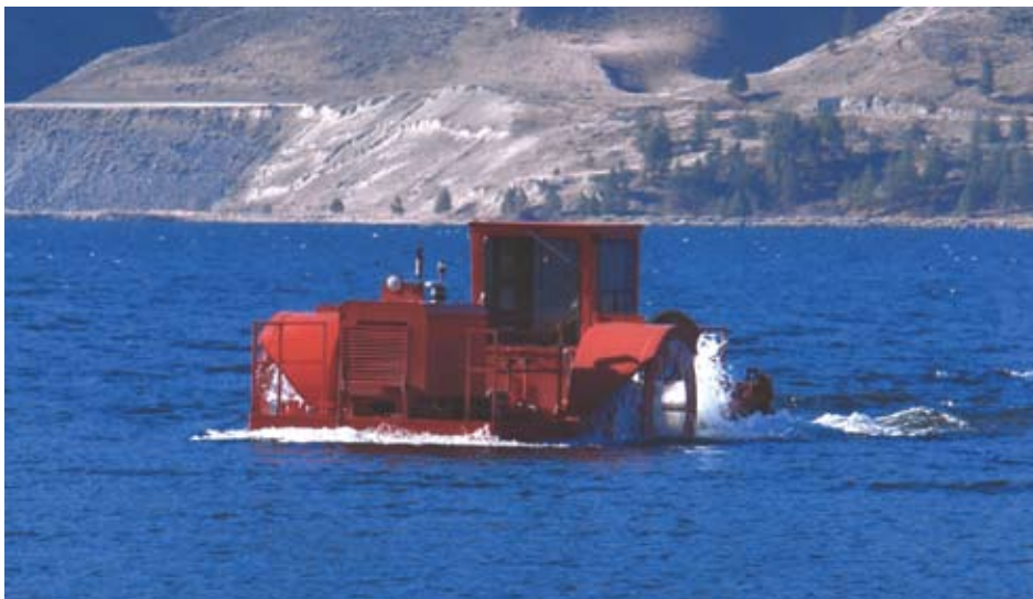
The machine used for rototilling Eurasian watermilfoil root systems on shallow portions of the lake floor.
