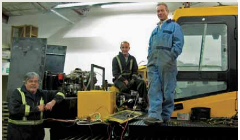
An extensive retrofit of the rubber-tracked crawler by the mechanically-inclined milfoil control crew enables the machine to de-root weed beds in areas too shallow for the floating rototillers to work.
