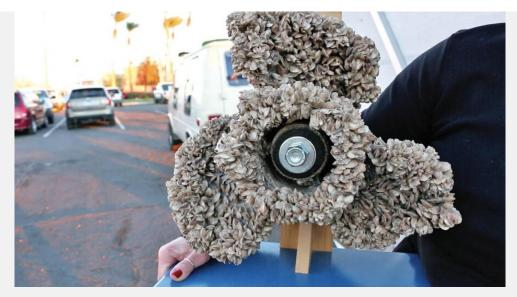
Mussels completely encrust a boat propeller in a still image from the short ducmentary Mussel Threat by Brynne Morrice. Zebra and quagga mussels will encrust any other surface in the water including water intakes, docks, boats, and power generation equipment. The razor-sharp shells also cover beaches, preventing people from going barefoot. (Photo supplied)
