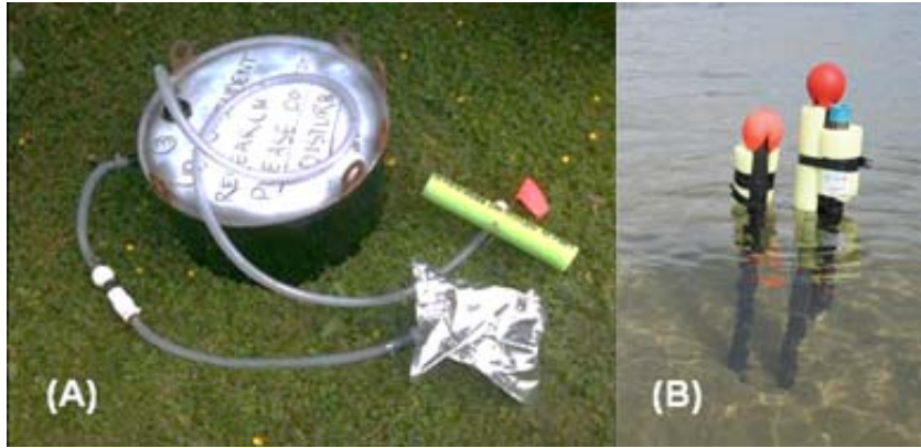
Figure 2.3 Physical measurement equipment: A) seepage meter (photo by N. Pyett), B) piezometer nest (photo by C. Baptie).
