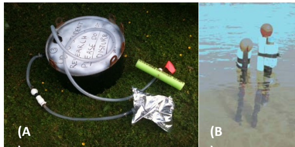
Figure 3: Apparatus used for groundwater discharge estimation: (A) Lee-type seepage meter, (B) piezometer nest used for hydraulic gradient measurement.
