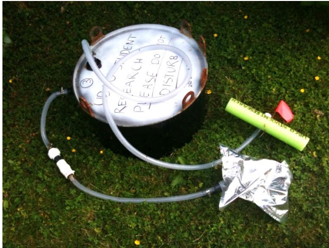
Figure A-1 A Lee-type seepage meter including the: A) vent line; and B) bag line
