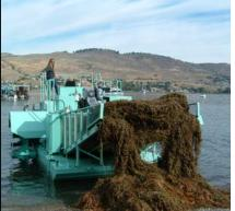
•Used during the summer to 'mow' dense Milfoil beds •Machine cuts to a depth of approximately 3 metres •Plant material is collected and transported to shore
