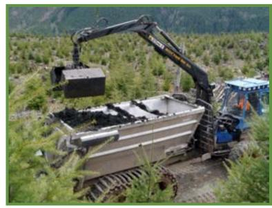
Biosolids forest fertilization (above). Significant increase in tree diameter can be seen in the tree rings after biosolids fertilization (left).
