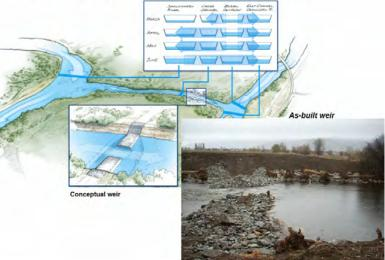
**Figure 2.14:** Okanagan River flow distribution weir.
