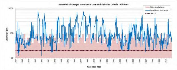
**Figure 2.3:** Historical Zosel Dam discharge relative to minimum recommended fish flow criteria, showing downstream fisheries flows frequently not being achieved, especially the years 2000 to 2010.
