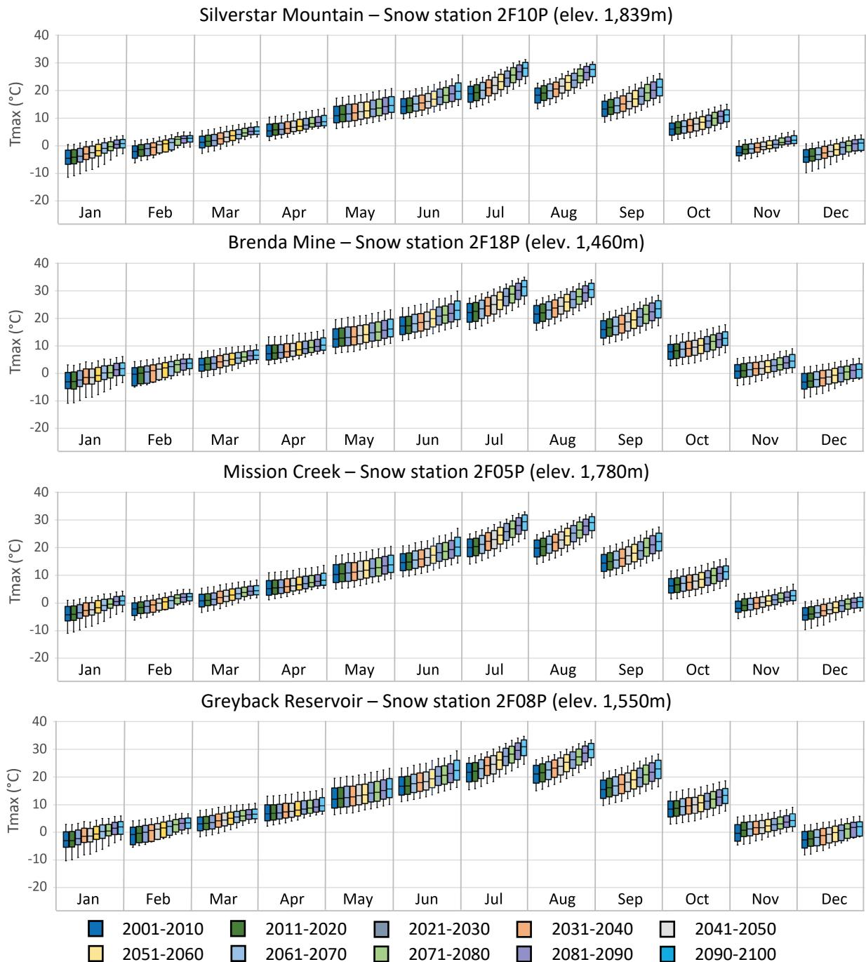
**Figure 2-11 Statistical distribution of projected daily maximum temperature, Tmax, in each decade for four snow stations in the Okanagan basin.**
