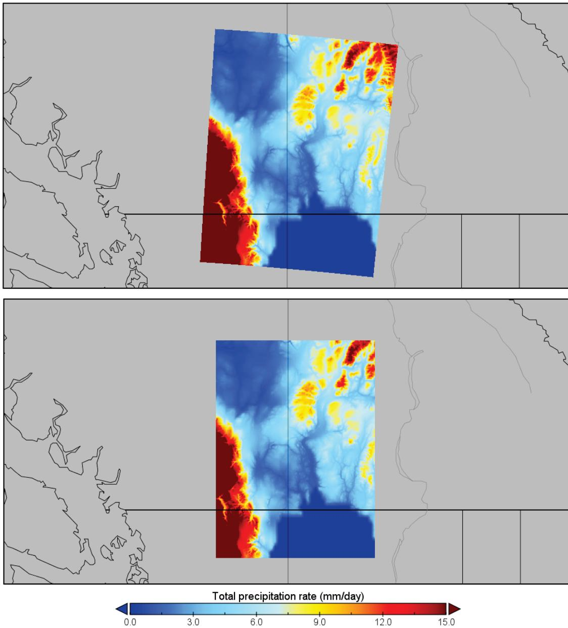
**Figure 2-5** Precipitation rates on example day January 4, 1945 in the original grid provided by AE (top panel) and resampled to a regular lat-lon grid (bottom panel). The three climatic variables, pr, tasmin and tasmax were resampled in this way.
