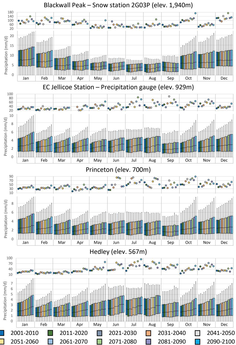
**Figure 2-18 Statistical distribution of projected daily precipitation in each decade for four representative locations in the Similkameen basin, covering a range of elevations. The vertical axis scale is different for the plots of maximum points above the boxplots.**
