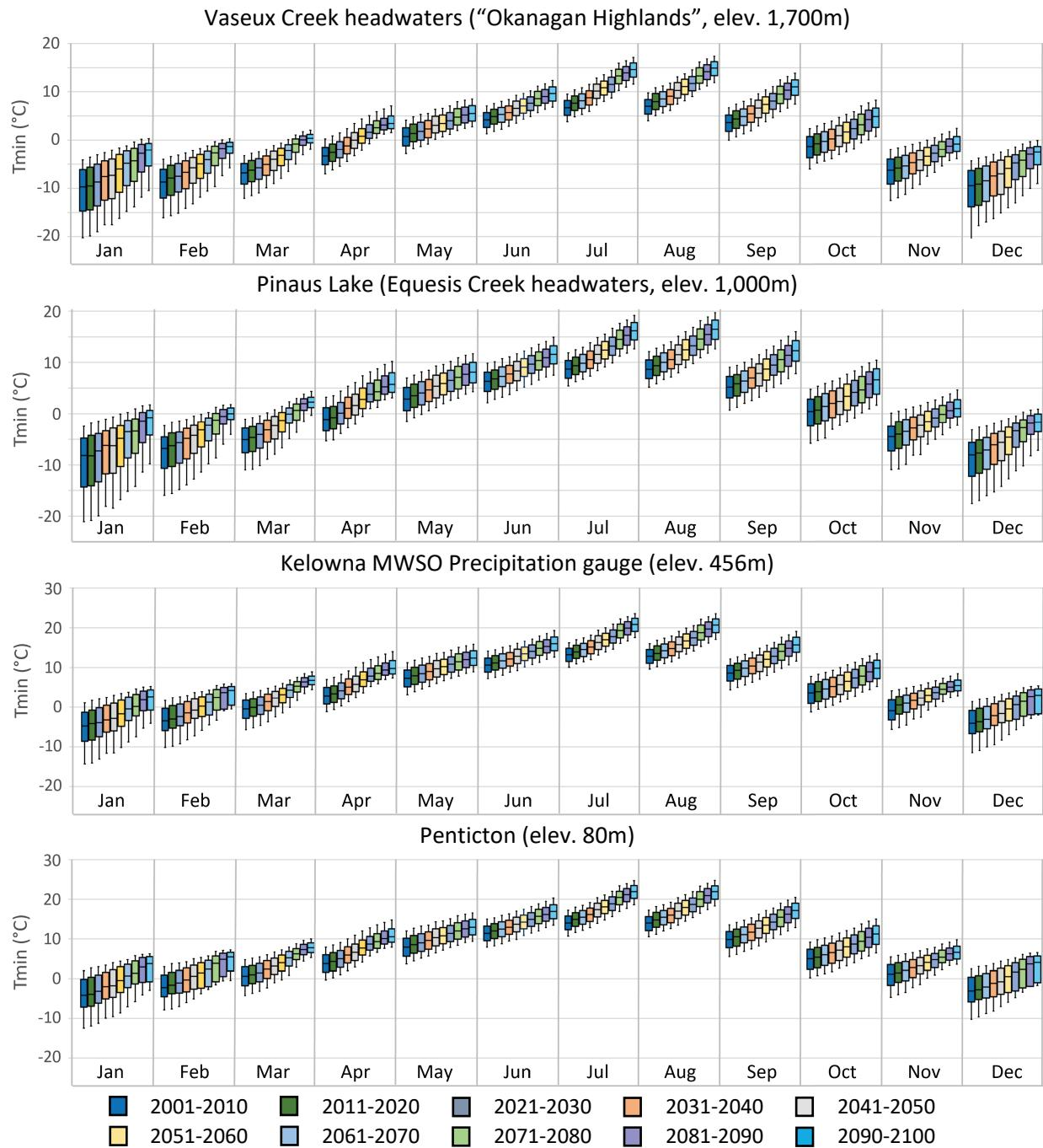
**Figure 2-9 Statistical distribution of projected daily minimum temperature,  $T_{min}$ , in each decade for four representative locations in the Okanagan basin, covering a range of elevations.**
