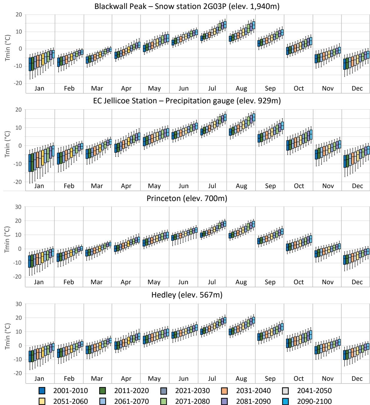
**Figure 2-10 Statistical distribution of projected daily minimum temperature,  $T_{min}$ , in each decade for four representative locations in the Similkameen basin, covering a range of elevations.**
