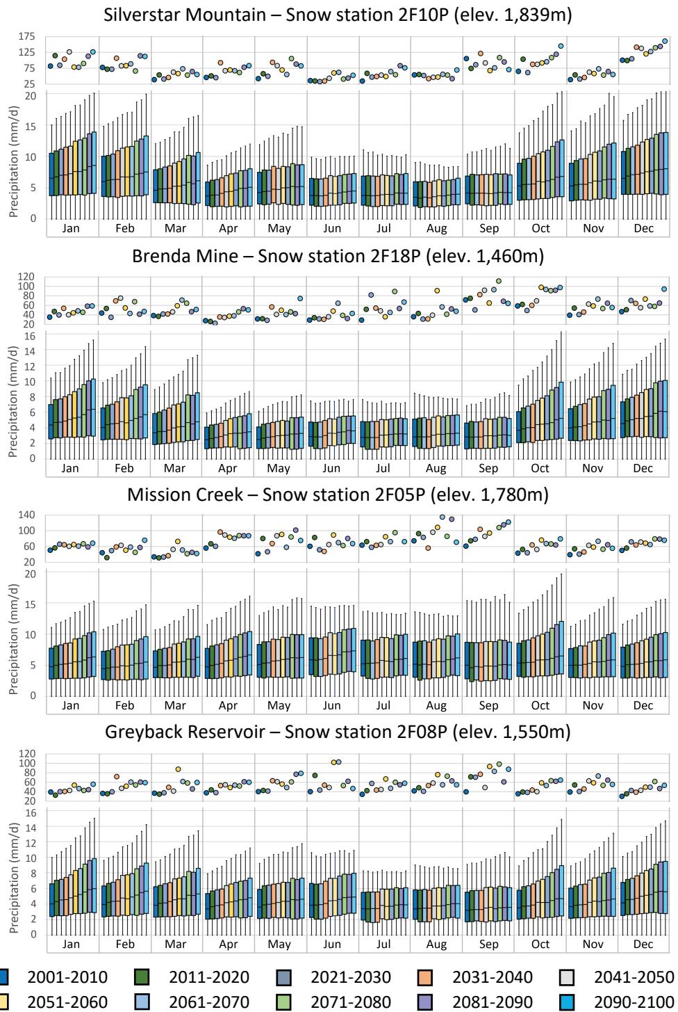
**Figure 2-16 Statistical distribution of projected daily precipitation in each decade for four snow stations in the Okanagan basin. The vertical axis scale is different for the plots of maximum points above the boxplots.**
