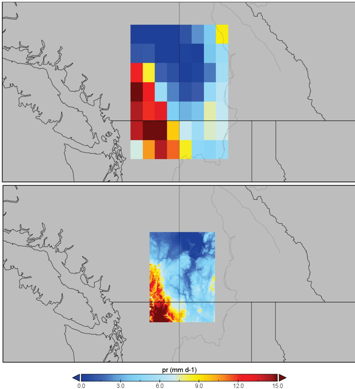
**Figure 2-6** Precipitation rate in the original CanLEADv1 data set (top panel) and statistically downscaled by the qdm algorithm of the ClimDown code (bottom panel).
