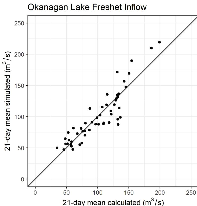
**Figure 3-13 Comparison of calculated and observed Okanagan Lake inflow. Values indicate mean 21-day inflow, at the day of the peak +/- 10 days. Black line is a 1:1 line.**
