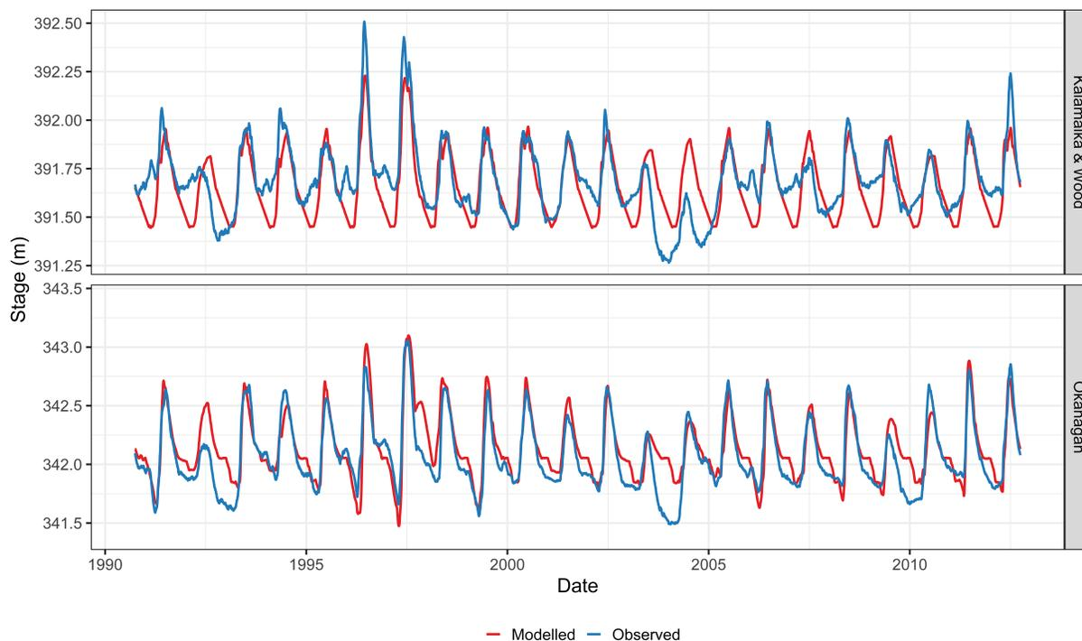
**Figure 3-10 Calibrated lake stages at Okanagan Lake and Kalamalka/Wood Lake.**
