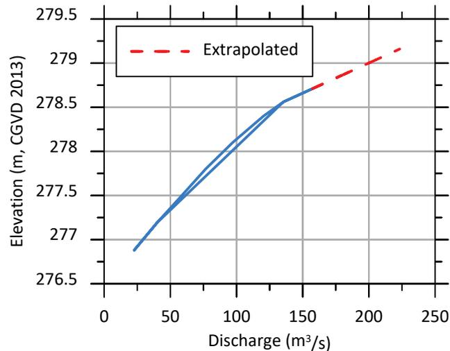
**Figure 3-17 Osoyoos Lake elevation-discharge rating, Zosel Dam with gates fully open (adapted from Summit [2010]).**
