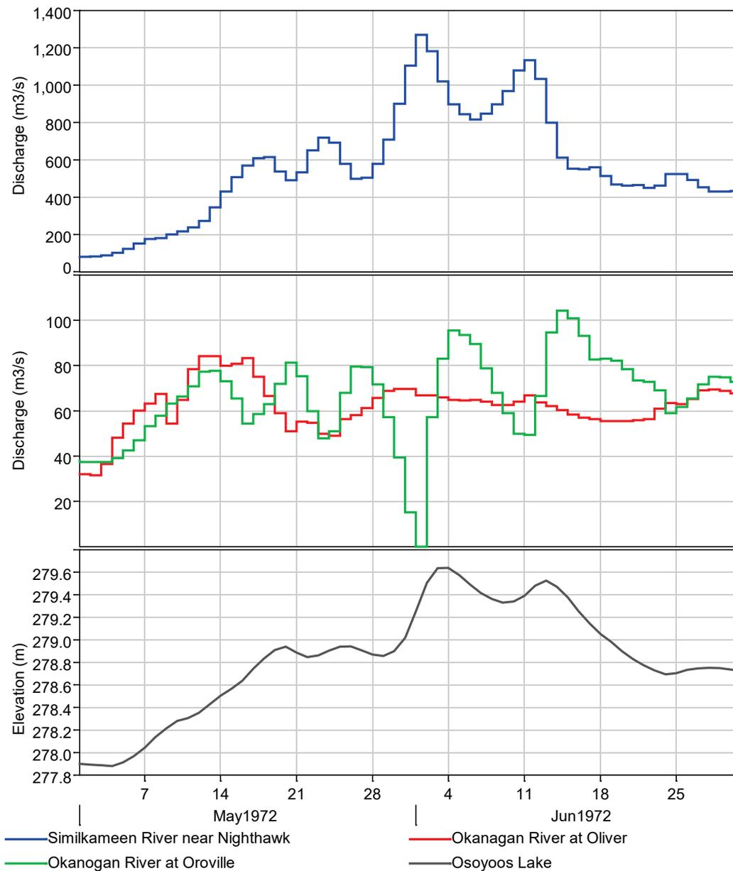
**Figure 3-16 Illustration of backwater effects from high Similkameen River flows in the 1972 freshet.**
