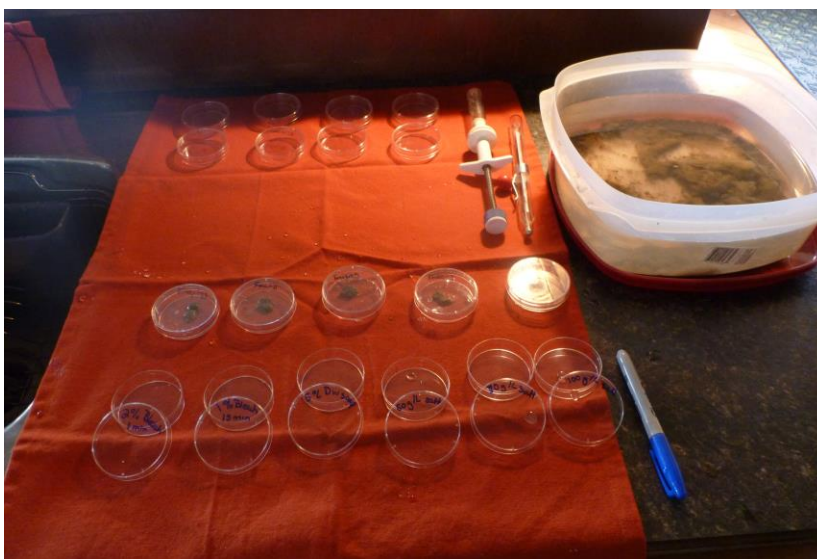
Figure A1.2 Sampling equipment lay-out for the Didymo trials
