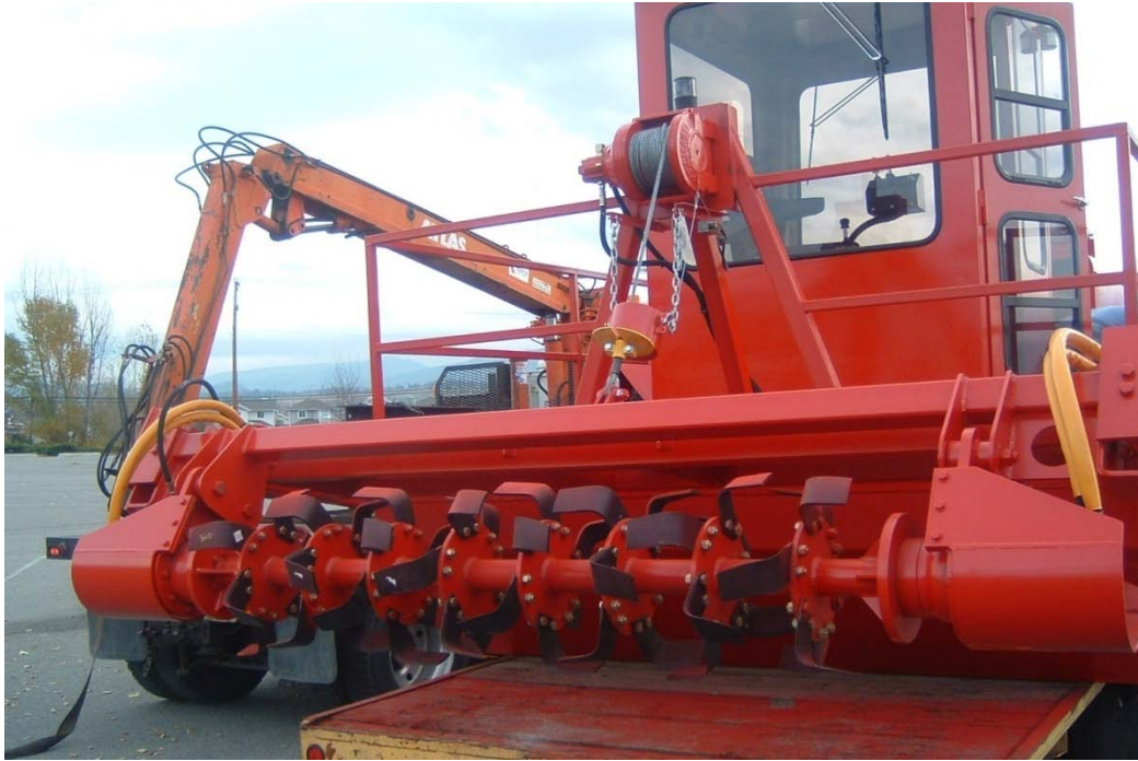
Figure 4: Rototiller from side, showing paddlewheels toward bow and enclosed cab at stern and rototiller from rear showing rototiller blades at stern of machine
