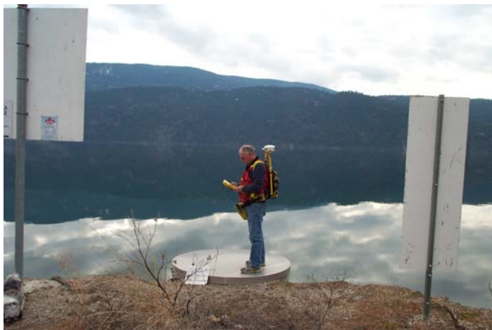
Figure 3. Capturing a differential GPS measurement at Kekuli Bay Provincial Park.
