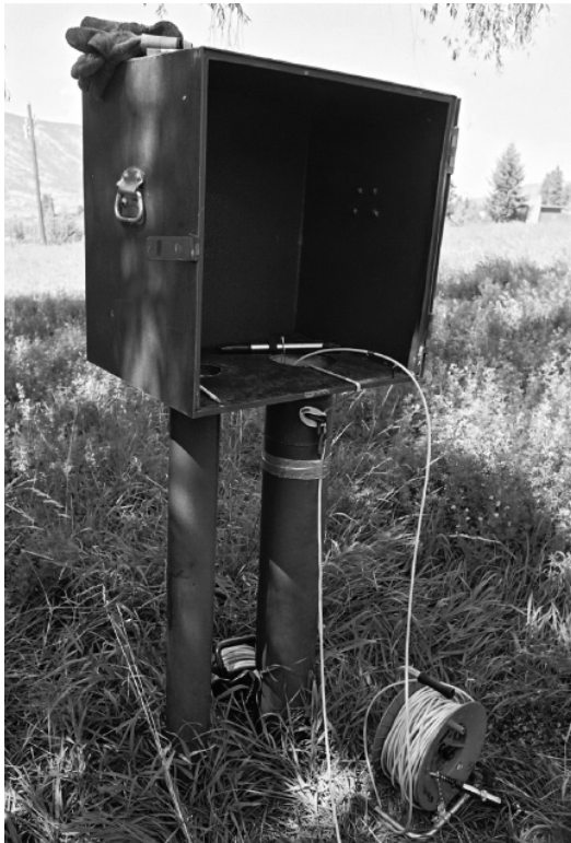
Figure 4. An observation well with a protective housing at the top of the casing. A slug test was in progress at the time the photograph was taken.
