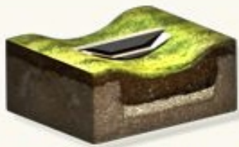
Infiltration Swale - Without Underdrain
