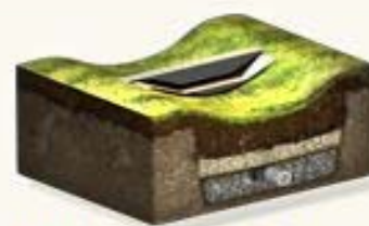
Infiltration Swale - With Underdrain
