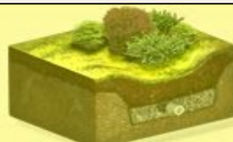
Rain Garden - With Underdrain
