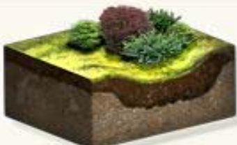
Rain Garden - Without Underdrain
