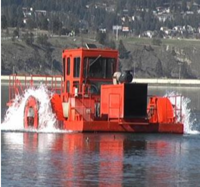
A milfoil harvester will be used to control an outbreak of the weed in Osoyoos Lake. (File Photo: Wayne Moore - Castanet)
