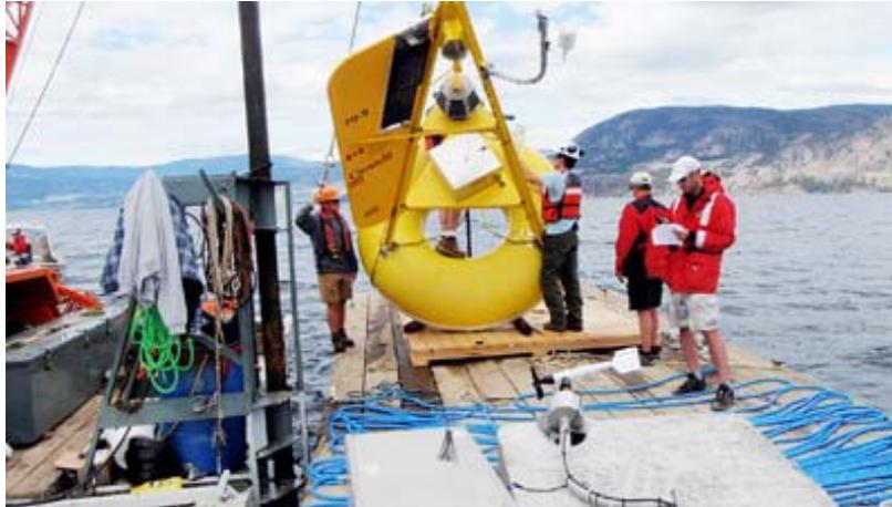
Environment Canada staff prepare to place one of three computerized buoys in Okanagan Lake which will be used to measure water evaporation levels in different weather conditions over the next three years.
