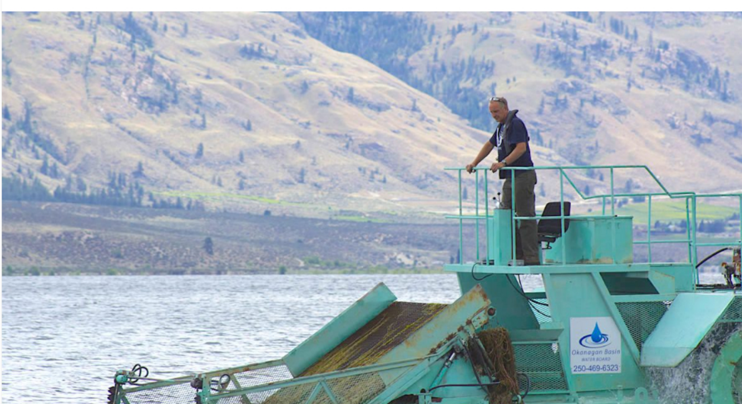
A current-generation milfoil harvester on Okanagan Lake. OBWB photo
