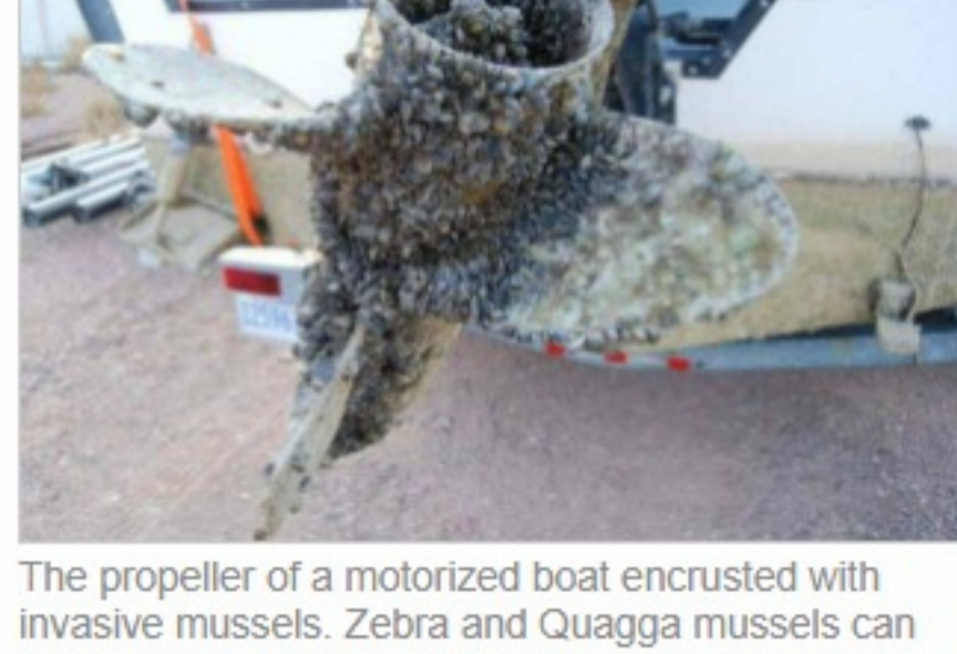
The propeller of a motorized boat encrusted with invasive mussels. Zebra and Quagga mussels can thrive in tiny crevices and even inside outboard motors, meaning very thorough cleaning is required to prevent their spread. (Contributed)
