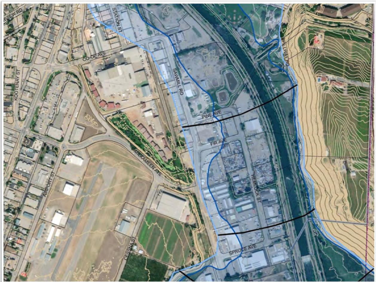
Figure 2. Fictional flood map for map design purposes only. Features include Orthophoto (faded), contours, property boundaries, flood extent with and without freeboard.
