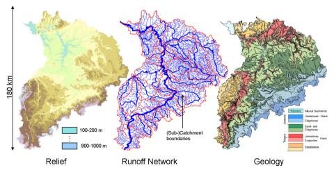
Fig. 2 Heterogeneities of relevant surface- and subsurface features at the *regional scale* (or *catchment scale*), using the Neckar catchment (14,000 km<sup>2</sup>) as an example (data provided by the state geological survey and environmental agency of the federal state of Baden Württemberg, Germany). Note the almost negligible extend of alluvial formations
