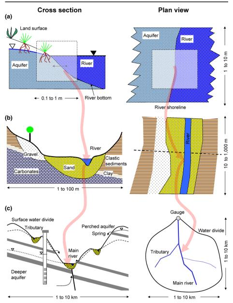
Fig. 1 Schematic representation of a the *point scale* (or *plot-scale*). Only influent conditions are shown, b the local scale (or reach scale), c the sub-catchment scale (or small catchment scale). The system may include different surface water reaches, different hydrostratigraphic units and different types of aquifers
