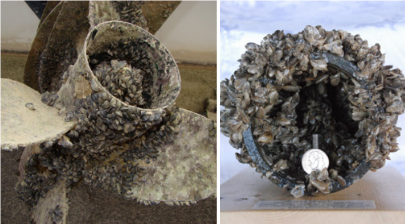
LEFT: Quagga mussels on rotor. RIGHT: Example of invasive mussel-infested pipe.
