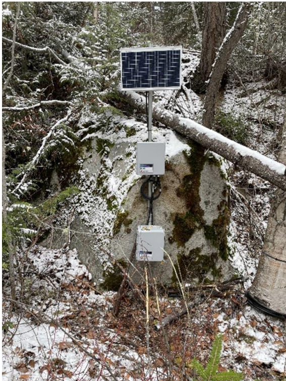
Photo above: Installation of Hydrometric Station at Naswhito Creek above Pumphouse.
