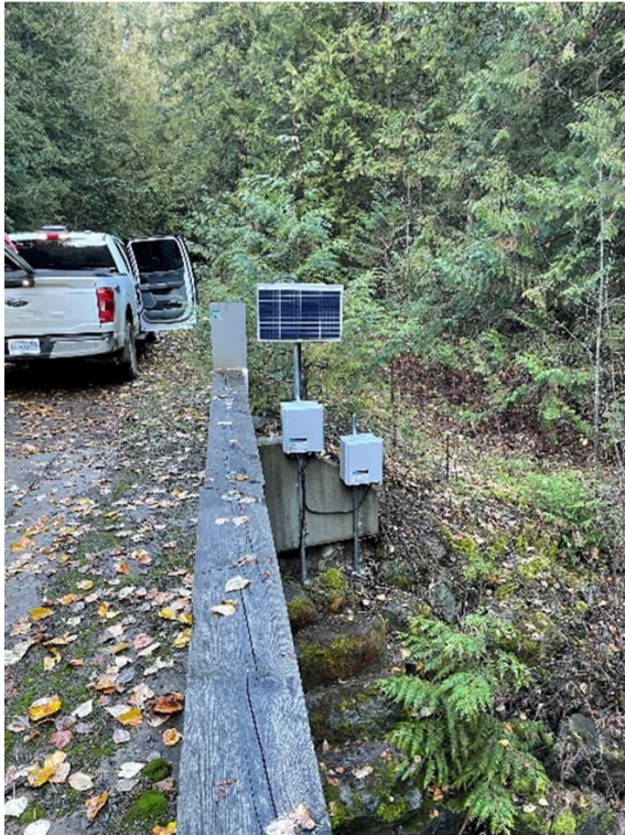
Photo above: Hydrometric Installation at Ewer Creek at Siwash Rock Main Bridge
