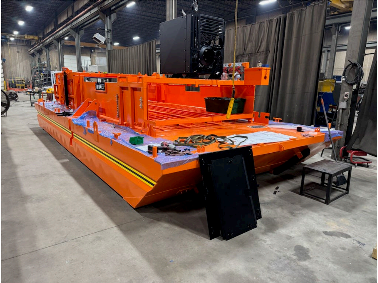
New Aquarius Systems HM-620 Custom Plant Harvester being assembled in North Prairie, Wisconsin. Capacity 15.5 cubic yards.
