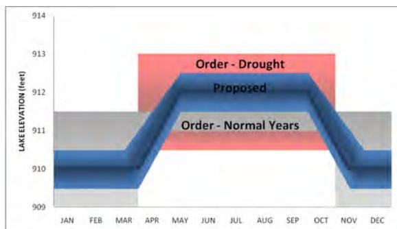
**Figure 4.1:** Recommended Osoyoos Lake elevation management plan (blue).
