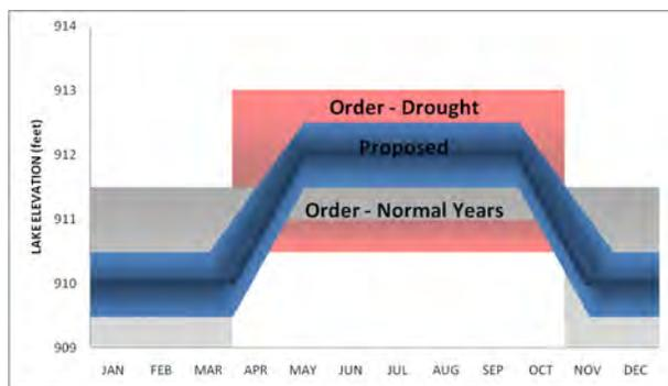
**Figure 2.4:** Recommended Osoyoos Lake elevation management plan (blue).
