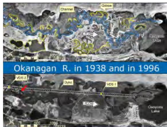
**Figure 2.17** The meandering Okanagan River in 1938 compared to the channelized river in 1996.
