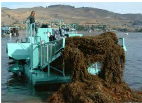
**Figure 2.10:** A harvester is used to mow watermilfoil plants in the Okanagan Valley mainstem lakes in the summer.
