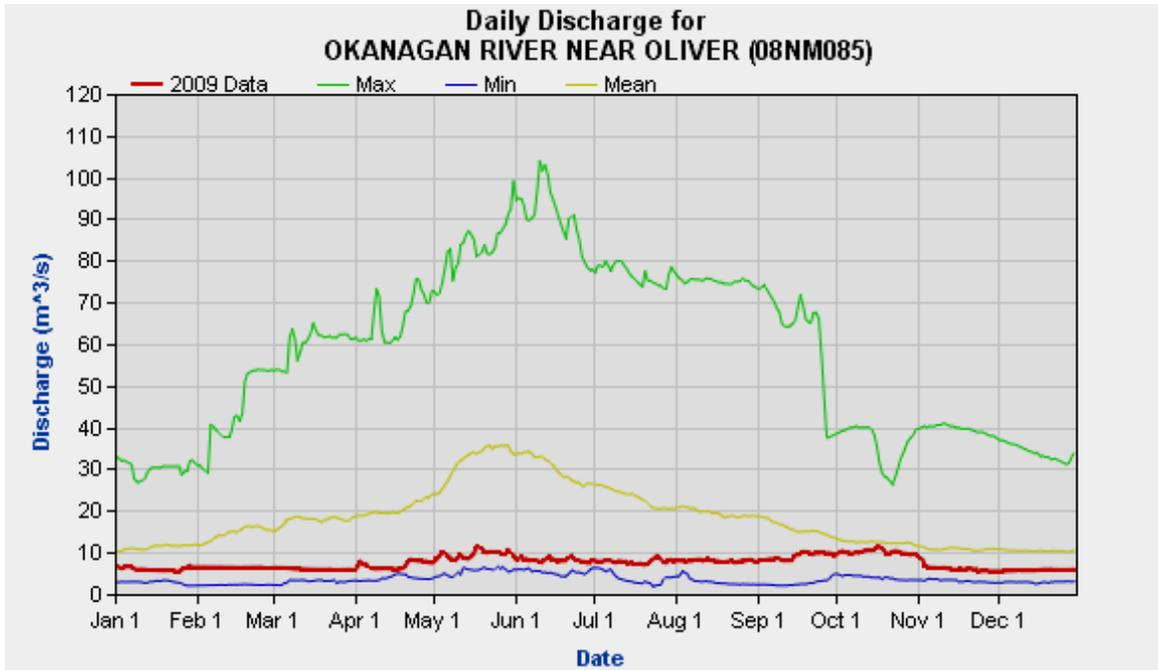
Figure 3. Minimum, maximum, and average daily discharge for Okanagan River near Oliver (Water Survey Canada station 08NM085).
